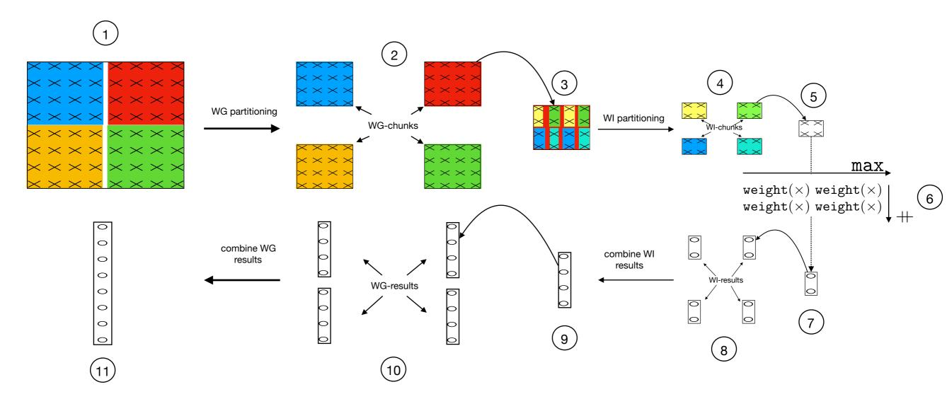
We exploit the algebraic representation of PRL to split the input data for WGs and WIs..
